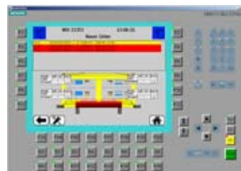
Fig 2. The elaboration of the measurement data into numbers. It contains the value reached at the pre-print, and the final value for the flaring position.
